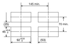
Normal Allowable Deviation=± (Value of JIS B 0401-1999 tolerance grade IT18) /2
